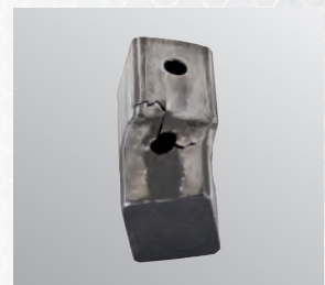
OTHERS: Uncontrolled breakaway can damage other components
